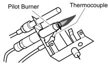
Figure 25 - Correct Pilot Flame Pattern
